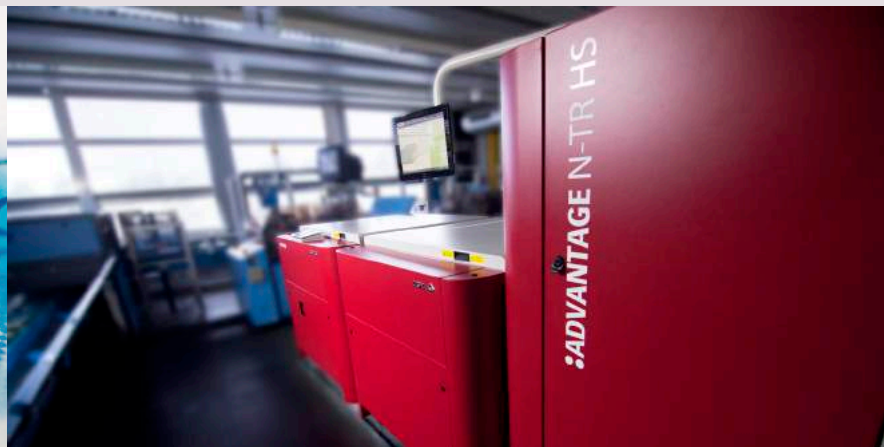
High-volume plate production system Advantage N-TR HS complete with on-line Attiro VHS COU.
