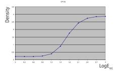
Machine processing 90 s 33°C (95°F) with G138i/G334i and CURIX Ortho Regular screen
