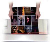
The Digitrim 64 can handle numerous types of media with a maximum thickness of 0.5mm (20 mil) including Polycarbonate, Laminates, Encapsulated Media, Photo Paper, Vinyl, Self-Adhesive Vinyl, PVC, Inkjet, Electrostatic Plotter Media, **Graphic Arts Film, Canvas and Duratrans.**
